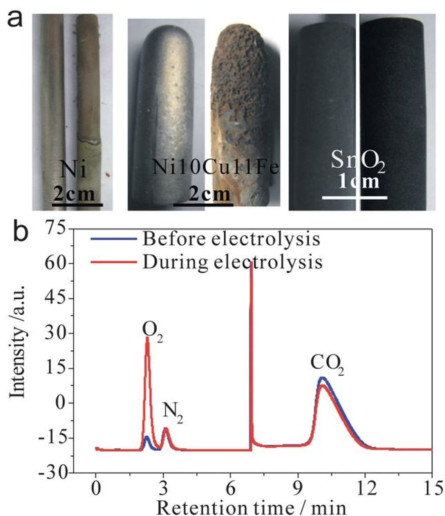
**Fig. 5** (a) Digital photos of Ni, Ni10Cu11Fe and  $\text{SnO}_2$  electrodes before and after serving as the anode under a constant cell voltage of 3.0 V in  $\text{Li}_2\text{CO}_3$ - $\text{Na}_2\text{CO}_3$ - $\text{K}_2\text{CO}_3$  melts at  $500^\circ\text{C}$  (2 hours for Ni and Ni10Cu11Fe anodes, more than 500 hours for  $\text{SnO}_2$  anode) and (b) gas chromatograms of the outlet gas before and during electrolysis (1 hour, 4.5 V cell voltage) using the  $\text{SnO}_2$  anode.
