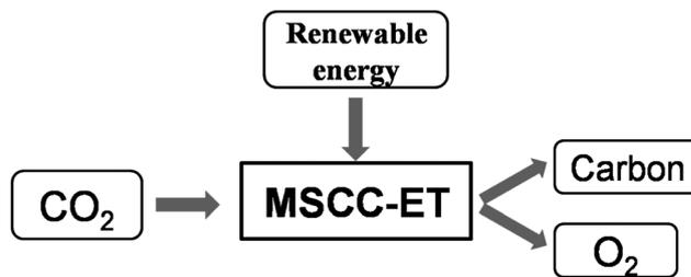
**Scheme 1** Schematic illustration of the Molten Salt CO<sub>2</sub> Capture and Electrochemical Transformation (MSCC-ET) process.
