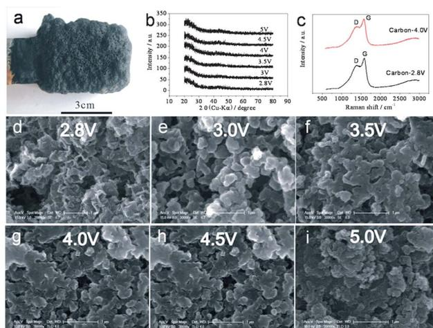
**Fig. 2** (a) Digital photo of a Ni cathode after 5 hours of electrolysis under 4.0 V cell voltage; (b) XRD patterns of the carbon deposited at the indicated cell voltages; (c) Raman spectra of the carbon obtained at 2.8 V and 4.0 V and (d–i) SEM images of the carbon obtained at the indicated conditions.
