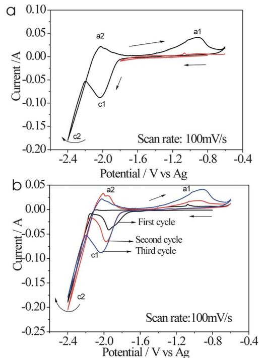
**Fig. 1** Cyclic voltammograms recorded from a Ni electrode in the molten Li<sub>2</sub>CO<sub>3</sub>–Na<sub>2</sub>CO<sub>3</sub>–K<sub>2</sub>CO<sub>3</sub> at 500 °C in the CO<sub>2</sub> atmosphere (a) in different potential ranges and (b) under consecutive cycling.
