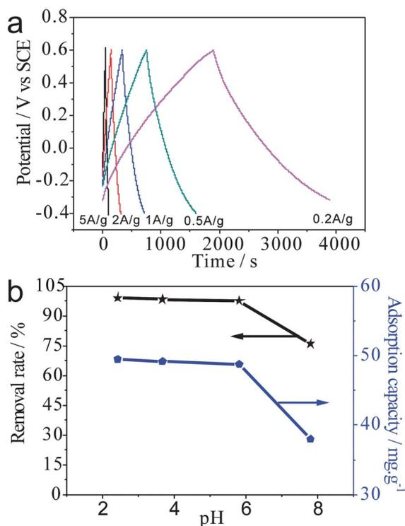
**Fig. 3** (a) Charge–discharge curves of the carbon material obtained at 4.0 V cell voltage in 1 M  $\text{H}_2\text{SO}_4$  aqueous solution and (b) adsorption capacity and the removal rate of  $\text{Cr}(\text{VI})$  by the carbon obtained at 4.0 V, the initial concentration of  $\text{Cr}(\text{VI})$  was  $50 \text{ mg L}^{-1}$ .
