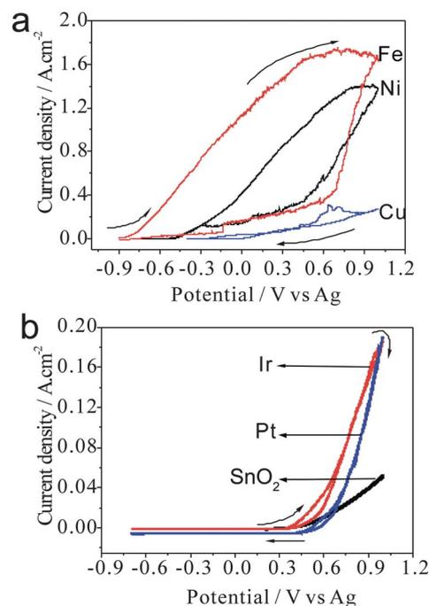
**Fig. 4** (a) Polarization curves of the Ni, Fe, Cu electrodes and (b) Pt, Ir,  $\text{SnO}_2$  electrodes in molten  $\text{Li}_2\text{CO}_3\text{--Na}_2\text{CO}_3\text{--K}_2\text{CO}_3$  at  $500^\circ\text{C}$  in the  $\text{CO}_2$  atmosphere, scan rate:  $5 \text{ mV s}^{-1}$ .
