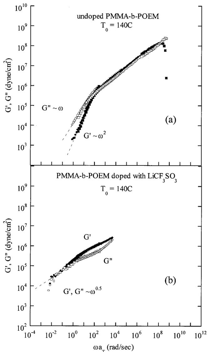
**Figure 2.** Master plots of  $G'$  and  $G''$  obtained about a reference temperature of  $140^\circ\text{C}$  for (a) undoped PMMA-*b*-POEM and (b) PMMA-*b*-POEM doped with  $\text{LiCF}_3\text{SO}_3$  (EO:Li<sup>+</sup> = 20:1).
