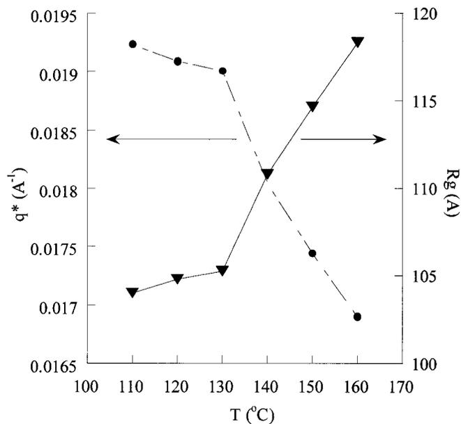
**Figure 5.** Temperature-dependence of the scattering peak position  $q^*$  and radius of gyration  $R_g$  for salt-doped PMMA-*b*-POEM (EO:Li<sup>+</sup> = 30:1).
