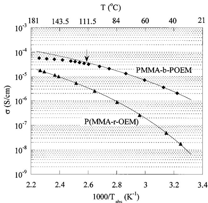
**Figure 7.** Ionic conductivity  $\sigma$  of salt-doped PMMA-*b*-POEM (diamonds) and P(MMA-*r*-OEM) (triangles) at a salt concentration of EO:Li<sup>+</sup> = 30:1. The full lines represent fits to the experimental data obtained with the VTF equation and using the parameters listed in Table II.
