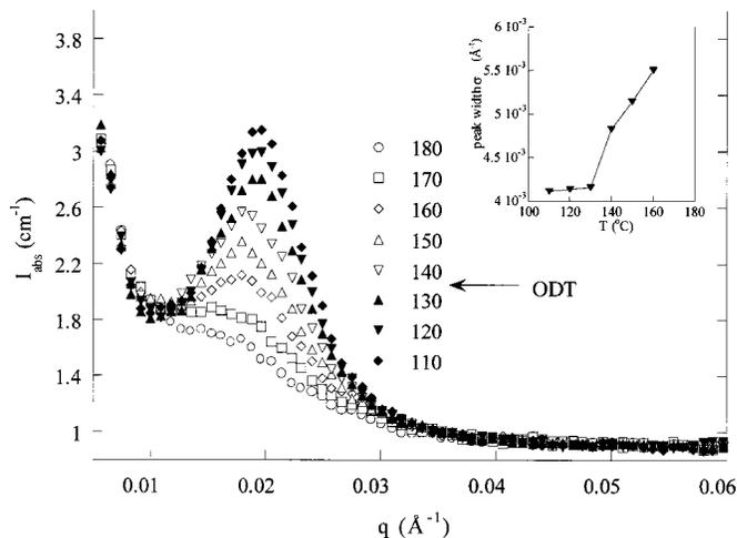
**Figure 4.** Scattering intensity profile as a function of temperature for PMMA-*b*-POEM doped with  $\text{LiCF}_3\text{SO}_3$  (EO:Li<sup>+</sup> = 30:1). The inset shows the change in peak width with temperature. Background subtracted intensity was fit to the Gaussian form  $I(q) = I_{\text{max}} \exp[-(q - q^*)^2/2\sigma^2]$  to extract  $q^*$  and  $\sigma$ .
