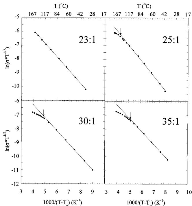
**Figure 8.** Linear conductivity plots for salt-doped PMMA-*b*-POEM as a function of temperature and at indicated salt concentrations. The full lines represent fits to the experimental data obtained with the VTF equation and using the parameters listed in Table II.
